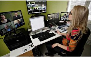
DESCRIPTION. We illustrate a setting for capturing multimodal data during multiperson interactions. In our lab, we simultaneously record electrodermal activity (EDA), heart rate, and respiration, synchronized with high-quality footage from a six-camera video system and microphones. High-resolution videos of faces facilitate the analysis of emotions through facial expressions, while videos capturing the entire body enable the study of movements and their synchronization.
