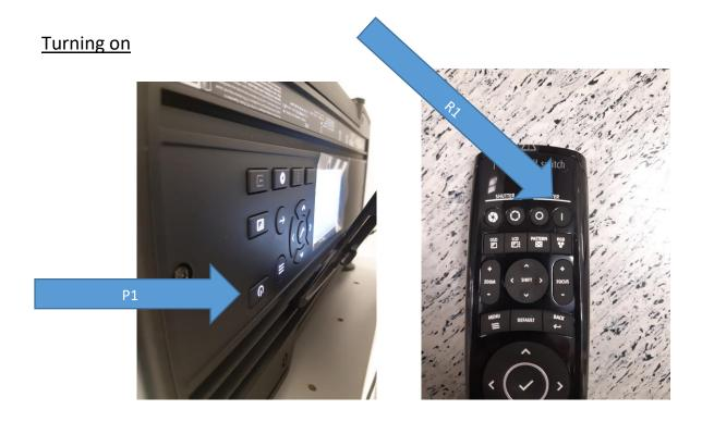
Press buttons (P1) or (R1) indicated in images above. The projectors power button will start blinking blue light. The power on sequence might take a minute or two. When the light is constantly showing blue, the projector is on.
