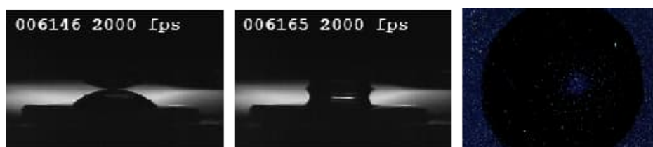
Figure 1. Left: High speed camera data of a sessile water droplet brought into contact with a silicon chip carrying a 2D deposit of multiwalled carbon nanotube (MWNT) material. Right: Optical micrograph of resulting imprint in the MWNT deposit.
