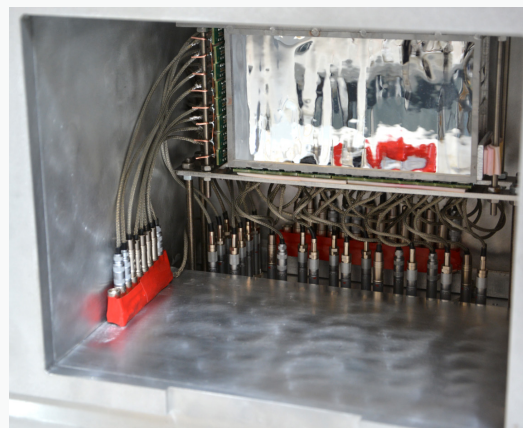
Detector in its place in the vacuum chamber. The active area dimensions are 14 \times 8 cm.
