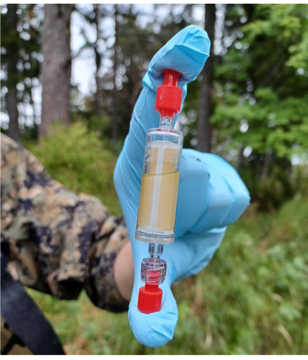
Fig. 3. Filter filled with DNA/RNA Shield to preserve eDNA.
