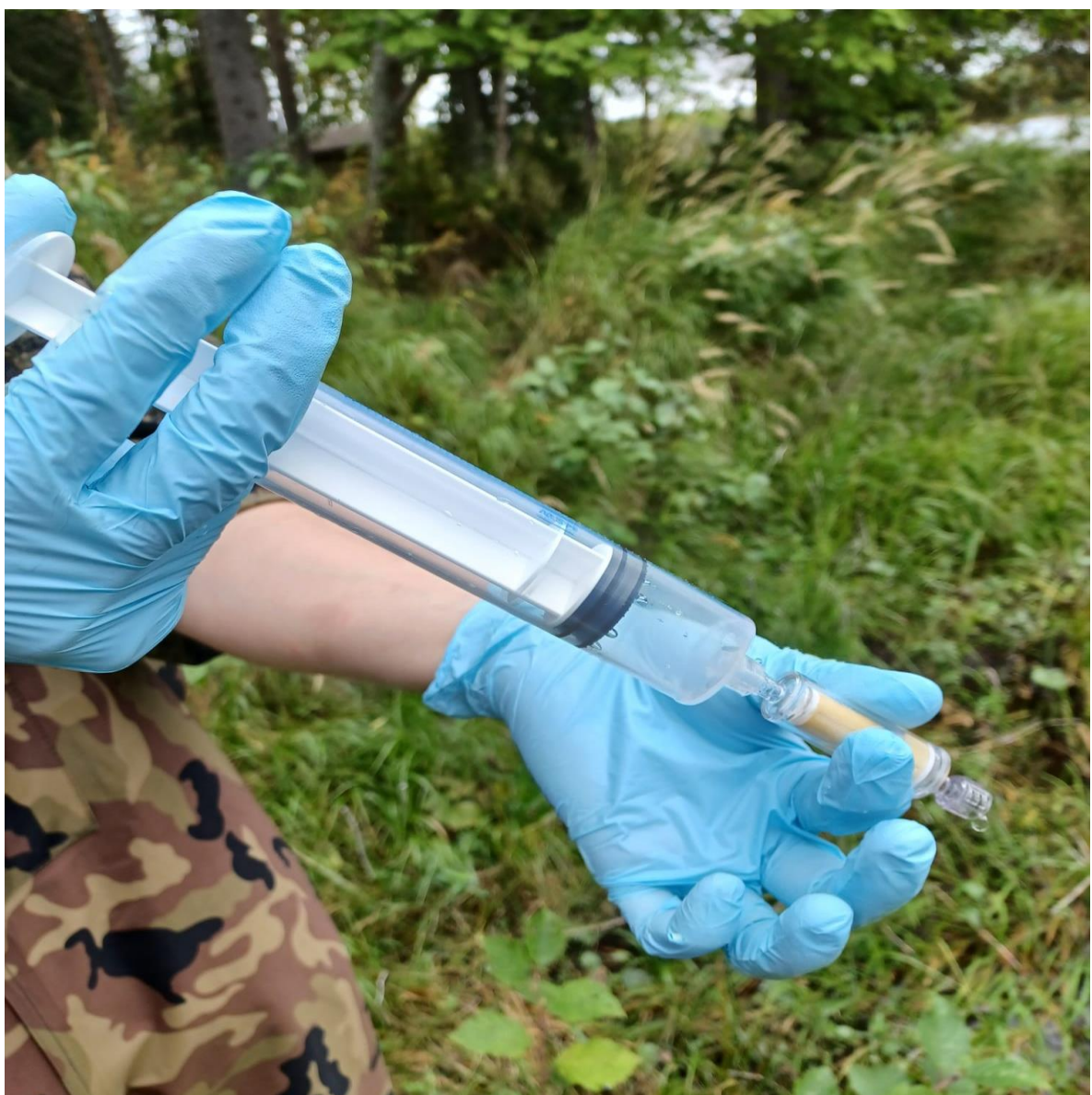
Fig. 2. Water samples pass through a filter to collect particles / eDNA.
