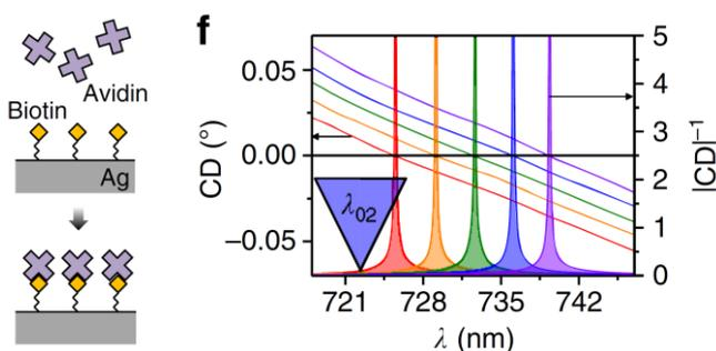
**Fig. 1.** Record refractive index sensitivity ( $1,091 \text{ nm RIU}^{-1}$  at  $\lambda = 921 \text{ nm}$ ) can be achieved by engineering the shapes and compositions of plasmonic nanoparticles. When coupled to a chiroptical detection scheme, background-free signal can be extracted with a high figure of merit (FOMs  $> 2,800 \text{ RIU}^{-1}$ ).<sup>[2]</sup>
