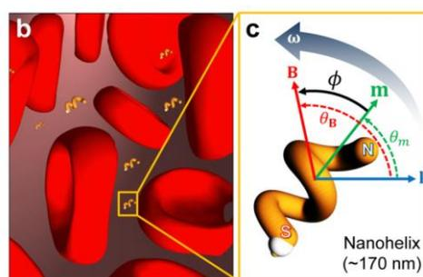
**Fig. 2.** Active nanorheology in full blood samples (up to 50% hematocrit) using chiral magnetoplasmonic nanoparticles. Nanoscale probes directly reveal blood plasma viscosity without interference of red blood cells. Background-free chiroptical signals can be detected in situ.<sup>[3]</sup>
