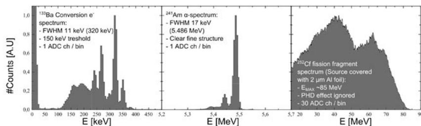
The spectra above were measured with a Micron DSSD connected to a Mesytech MPRT-16 preamp and Lyrtec/Nutaq digital electronics. All the measurements were made with the same settings, only varying
