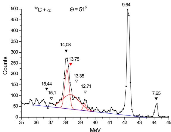
A sample spectrum of alpha-particles from the inelastic  $^{12}\text{C} + \alpha$  scattering at 65 MeV
