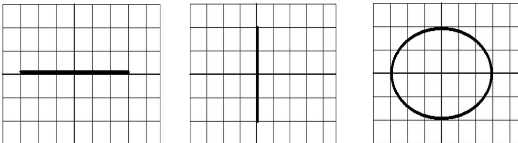
**Figure 3.** Principles of the XY mode: the signal of the second channel which is mapped on to y-axis is grounded (GD switch is on) and signal from another channel is shown parallel to x- axis. In the second picture, situation is reversed. In third picture, both signals are shown and they are mapped onto the same picture as a function of time.
