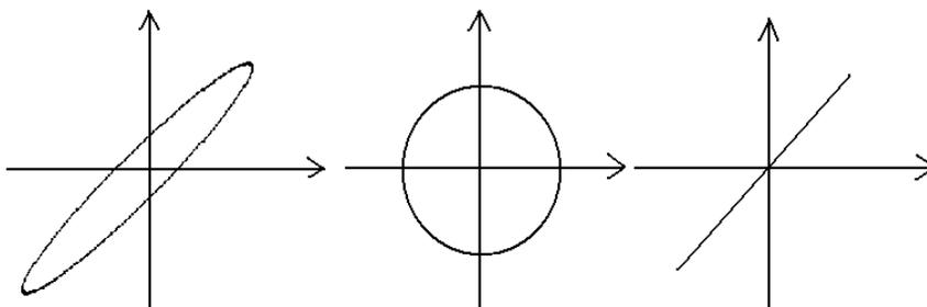
**Figure 6.** Some xy plots you might see on the scopes screen. In the picture left phase-difference is 45°, in middle 90° and to the right 0°.
