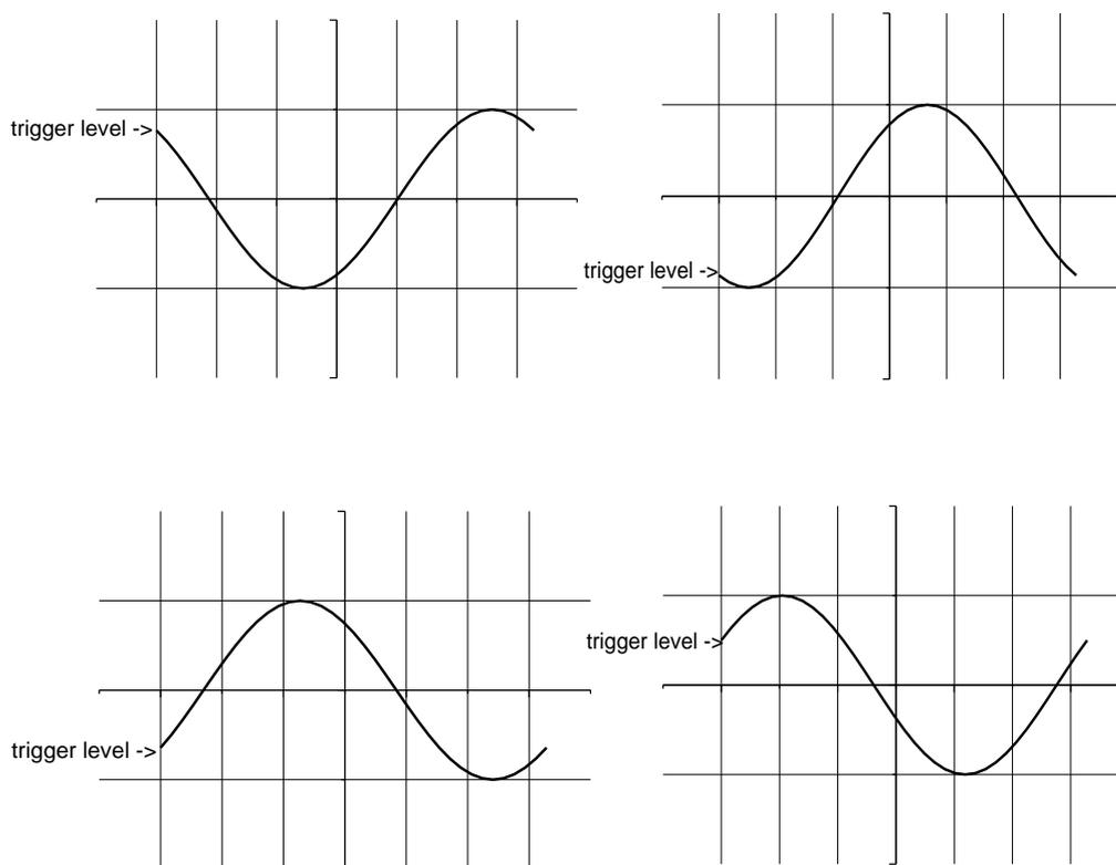
**Figure 2.** Pictures on the oscilloscope screen, when different LEVEL and SLOPE settings are used. Trigger is set on descending part (top) and ascending part (bottom) of the signal.
