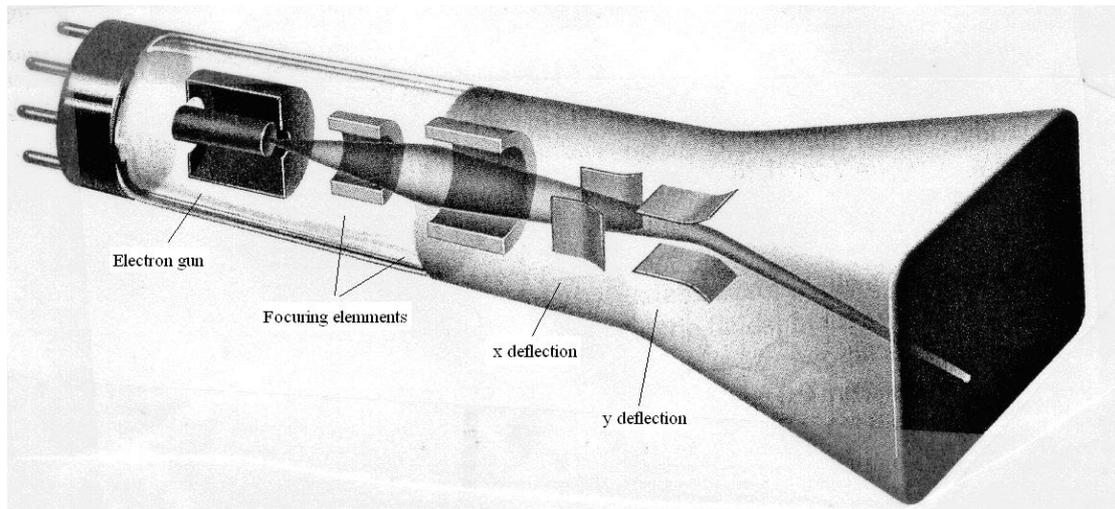
**Fig 1.** Main components of a cathode-ray tube
